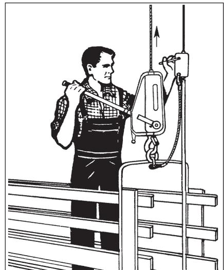
Fig. 6 - Releasing the BLOCSTOP whilst lowering the platform
