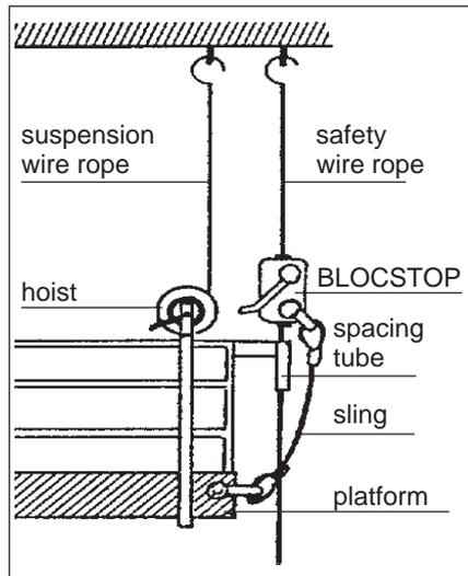
Fig. 5 - BLOCSTOP on safety wire rope
