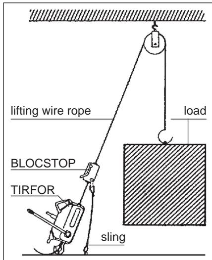
Fig. 4 - BLOCSTOP on lifting wire rope
